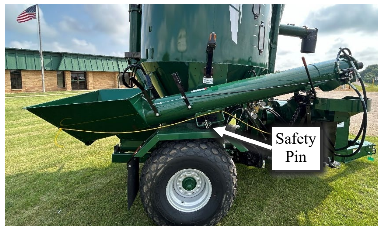
Figure 37 – Auger Feeder (Shown in Transport Position).
