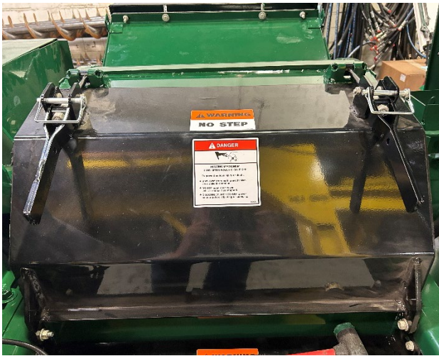
Figure 23 - Locking Pin and Latch on Hammer Mill Door.
