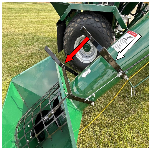
Figure 43 - Hydraulic Auger Feeder Controls (Shown in ON/RUN Position): Throttle Controls and Emergency Shutoff (Red Arrows).
