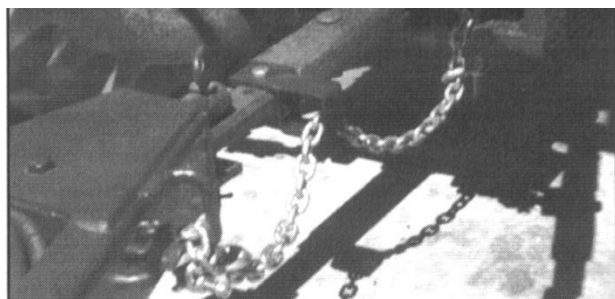
Figure 10 - Grinder Attached to the Tractor with Safety Chain.
