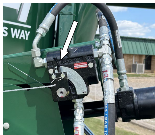
Figure 44 - Hydraulic Auger Feeder Control - Shown in Full ON/RUN Position (See Arrow).
