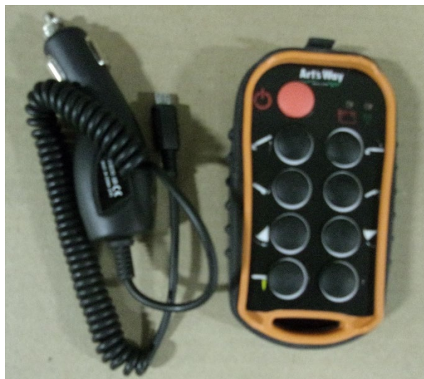
Figure 102 – Macro-Remote Control device with Charger.
