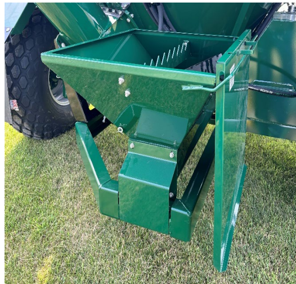
Figure 24 - Supplement Hopper Located on Center Rear Right Hand Side of Machine
