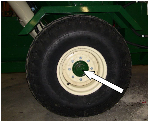
Figure 81 - Wheel Bearing Lubrication.
