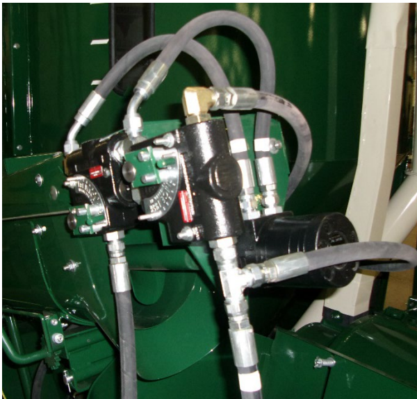
Figure 117 - Roll Feed and Auger Feeder Flow Control Valves.
