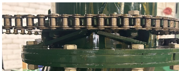
Figure 54 - Hydraulic Swing Adjustment (Shields Removed for Clarity).
