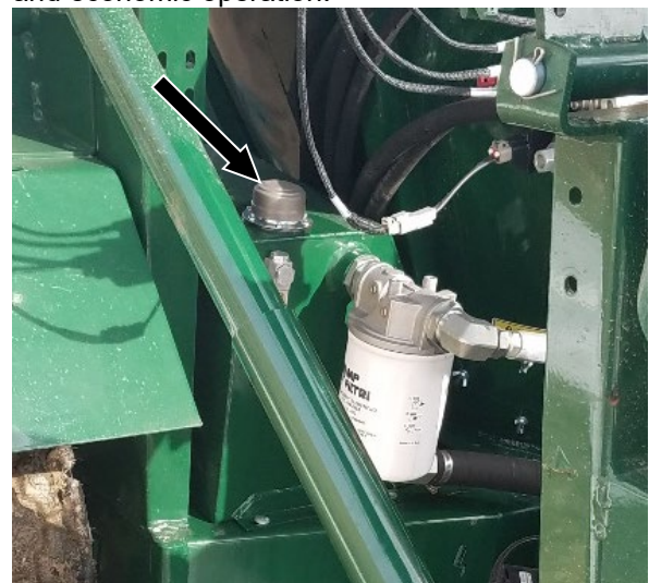
Figure 113a – Hydraulic Reservoir Cap (see Arrow)
