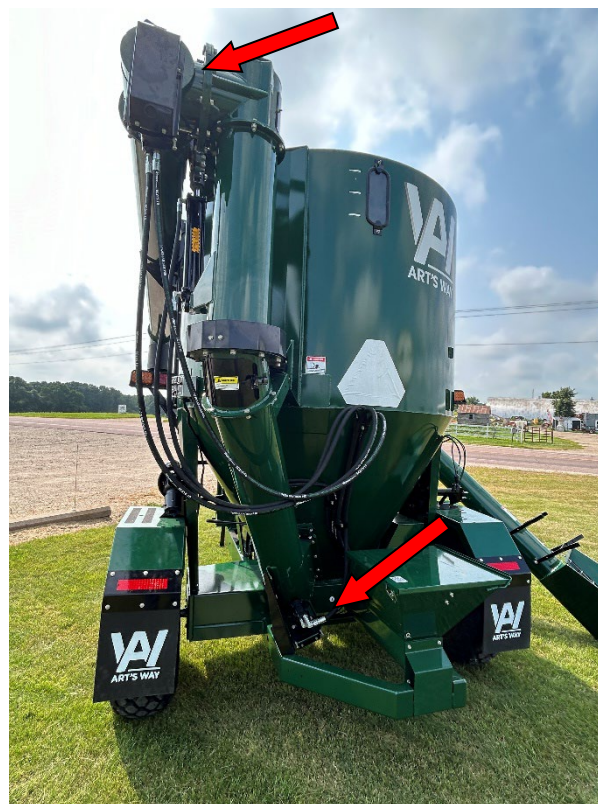
Figure 56 - Discharge Auger Drive Chain Locations (See Arrows).
