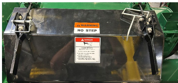
Figure 6 - Screen Hook Storage.
