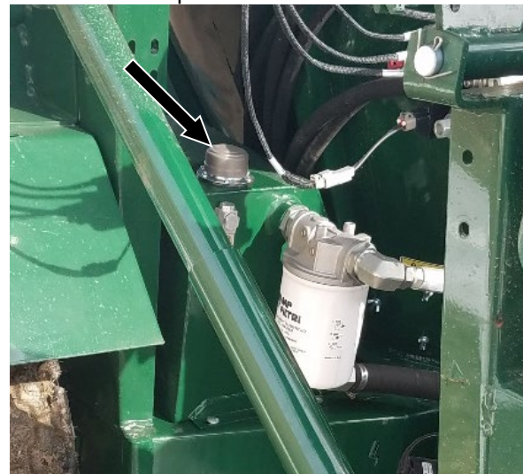
Figure 113a – Hydraulic Reservoir Cap (see Arrow)
