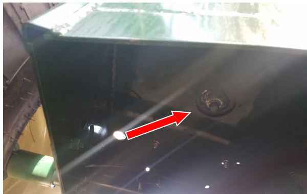
Figure 112 –Drain Underneath Reservoir Tank Base (Red Arrow).
