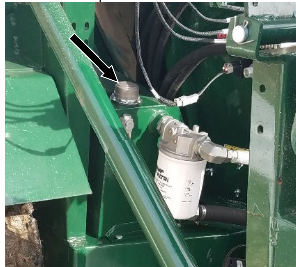
Figure 113a – Hydraulic Reservoir Cap (see Arrow)
