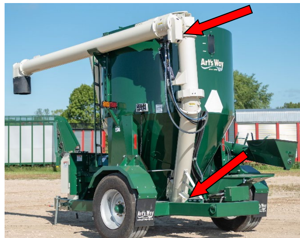
Figure 56 - Discharge Auger Drive Chain Locations (See Arrows).
