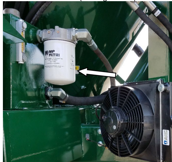
Figure 110 – Reservoir Filter (see Arrow)
