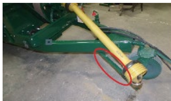
Figure 7a - PTO Driveline Storage Bracket.
