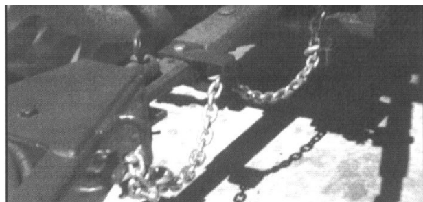
Figure 11 - Grinder Attached to the Tractor with Safety Chain.
