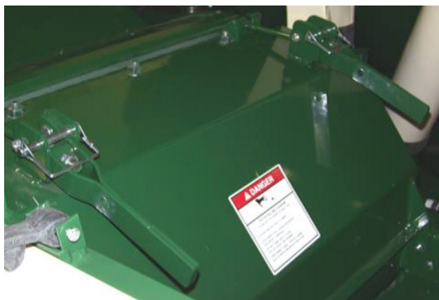
Figure 7 - Locking Pin and Latch on Hammer mill Door
