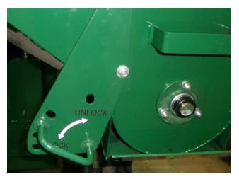
Figure 10 - Auger Feeder Latch Handle (Shown Locked)
