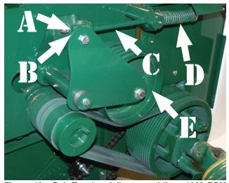
Figure 19 - Belt Tension Adjustment Idler - 1000 RPM Drive Shown
