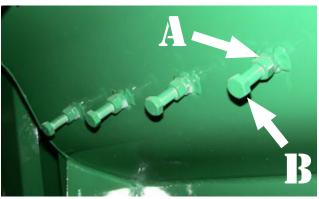
Figure 5 - Hay Retard Bolts (A - Lock Nut; B - Adjustable Retard Bolt, 26 Inch Hammer mill Shown)
