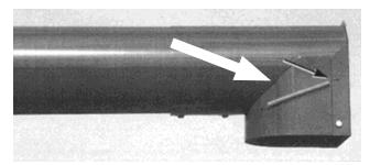
Figure 9 - Unloading Auger Hood
