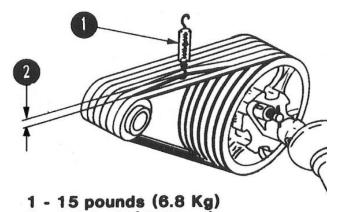
2 - 1/4 inch (.635 cm) Figure 21 - Checking Belt Tension
