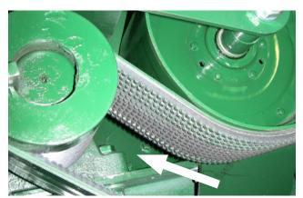
Figure 39 - Hammer mill Removal Hole, Plate To Be Removed
