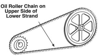
Figure 31 - Oiling Roller Chains
