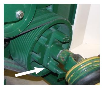
Figure 29 - Hammermill Clutch Pin
