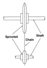
Figure 35 - Sprocket Alignment
