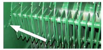
Figure 38 - Hammer Removal Inside Hammer mill, Hole to Remove Hammer mill Rods
