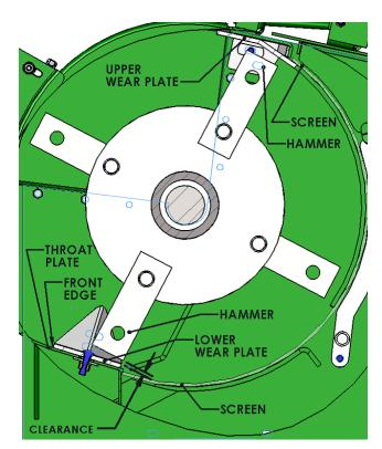
Figure 4 - Wear Plate Detail
