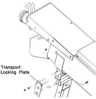
Figure 15 - Transport Locking Plate
