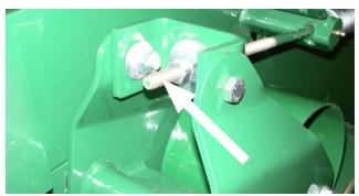
Figure 40 - Belt Replacement, Idler Roller
