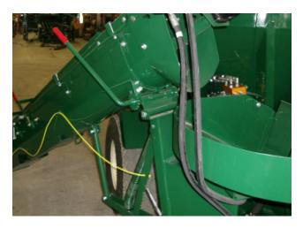
Figure 13 - Auger Feeder Positioner And Spring Adjustment
