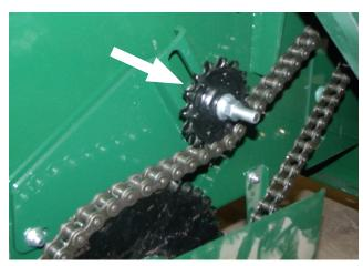
Figure 18 - Mill to Auger Drive Chain
