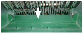
Figure 3 - Lower Wear Plate at Throat of the Hammermill
