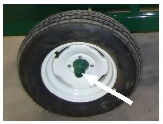
Figure 33 - Wheel Bearing Lubrication
