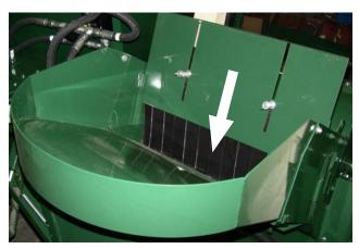
Figure 2 - Feed Gate at Throat of the Hammermill
