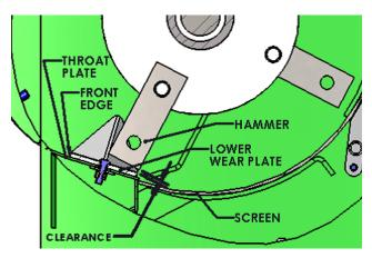
Figure 43 - Lower Wear Plate Detail
