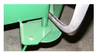
Figure 12 - Auger Feeder Swing Brake
