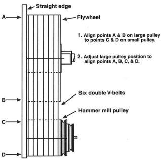
Figure 22 - Belt Pulley Alignment
