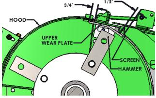
Figure 42 - Upper Wear Plate Detail
