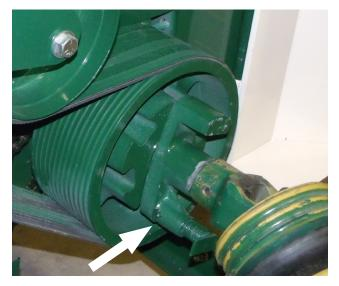
Figure 1 - Hammermill Clutch Pin
