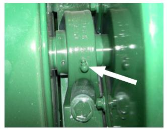
Figure 27 - Rear Cylinder Shaft Bearing
