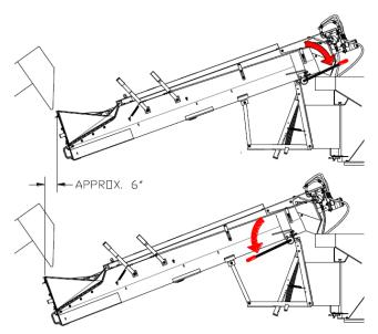
Figure 14 - Auger Feeder Positioner operation
