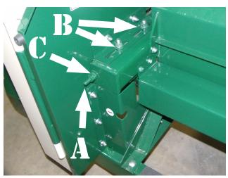
Figure 20 - Belt Tension Adjustment Bearing Mount
