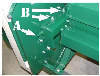
Figure 41 - Belt Replacement, Drive Sheave and Bearing Mount
