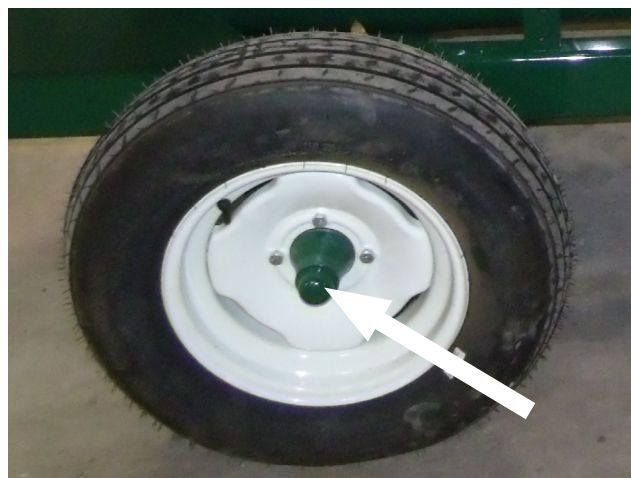
Figure 33 - Wheel Bearing Lubrication
