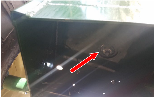
Figure 98 – Drain Underneath Reservoir Tank Base (Red Arrow).
