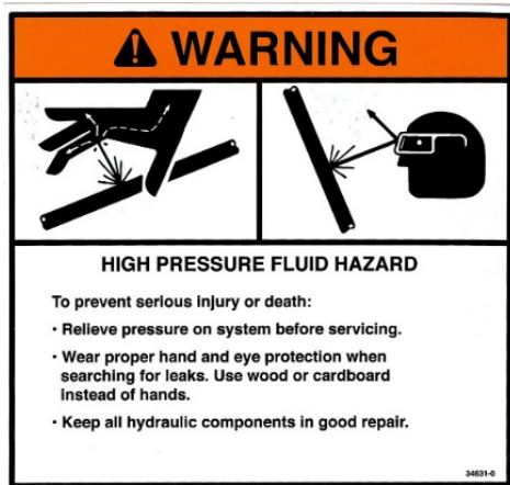
8. WARNING – High Pressure Fluid Hazard (346310)
