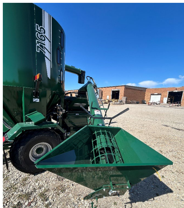
Figure 8 - Model 7165 Cattlemaxx with Self-Contained Hydraulics, Auger Feeder.
