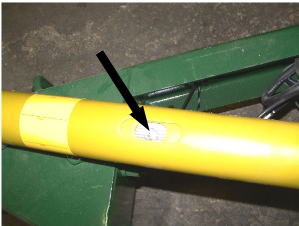
Figure 59 - PTO Driveline Shaft (See Arrow).
