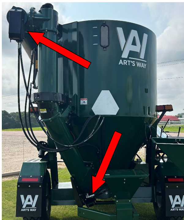
Figure 52 – Discharge Auger Drive Chain Locations (see arrows).
