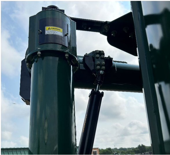
Figure 27 - Unloading Auger Positioning (Shown in Upper 60° to -11° Configuration).
