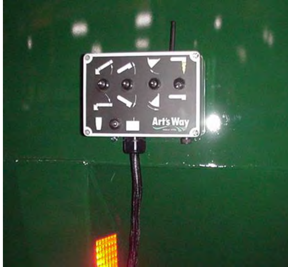
Figure 99 – Complete Control Box with Internal Receiver as Backup Remote Control Box Mounted on Left Rear Side of Mixer Tank (for Functions see Figure 104).
