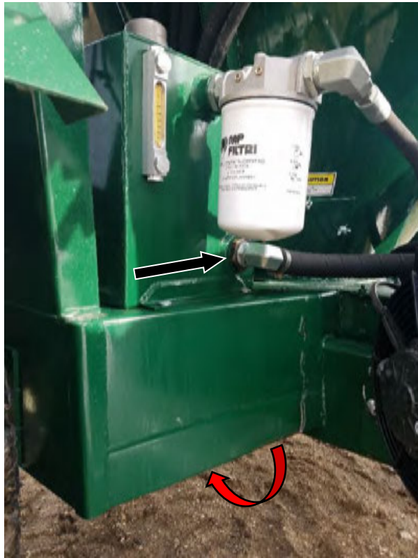
Figure 111 – Reservoir Strainer (Black Arrow) and Drain Underneath Base Plate (Red Arrow).
