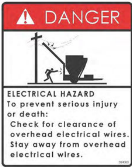
7. DANGER – Electrocutation Hazard (384000)
