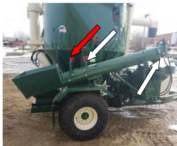
Figure 43 - Hydraulic Auger Feeder Controls (Shown in ON/RUN Position): Throttle Controls (White Arrows) and Emergency Shutoff (Red Arrows).
