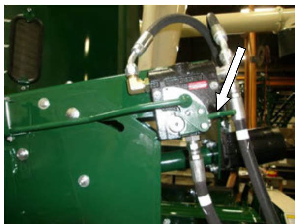
Figure 44 - Hydraulic Auger Feeder Control - Shown in Full ON/RUN Position (See Arrow).
