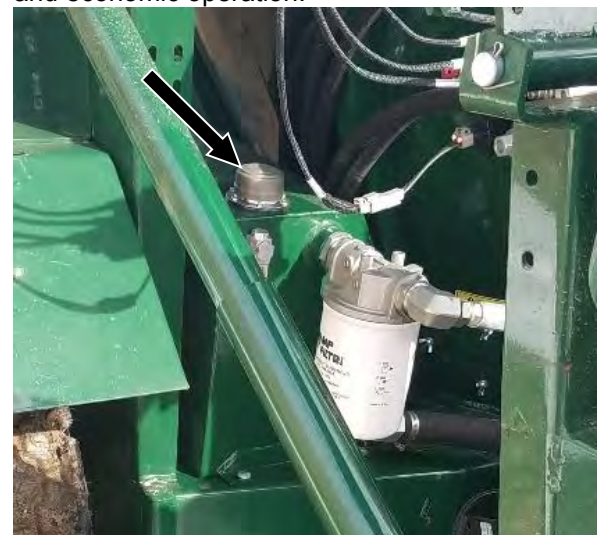
Figure 113a – Hydraulic Reservoir Cap (see Arrow)
