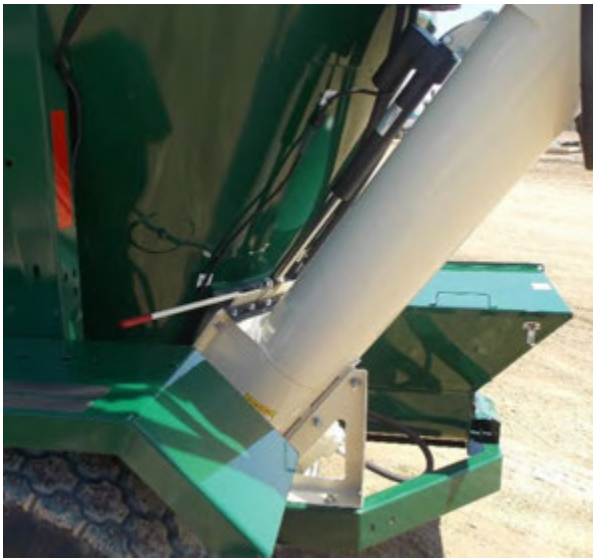
Figure 31 - Discharge Gate with Electric Actuator in Closed Position.
