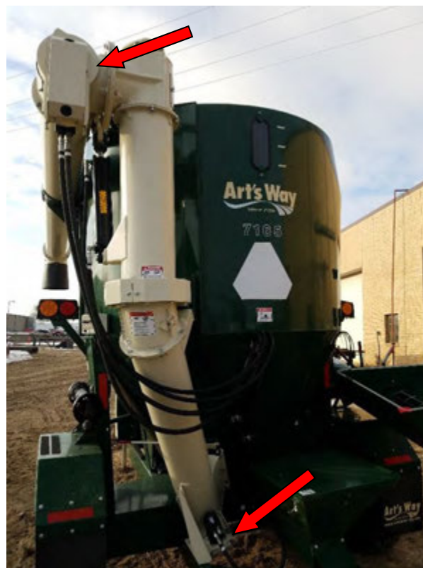
Figure 56 - Discharge Auger Drive Chain Locations (See Arrows).
