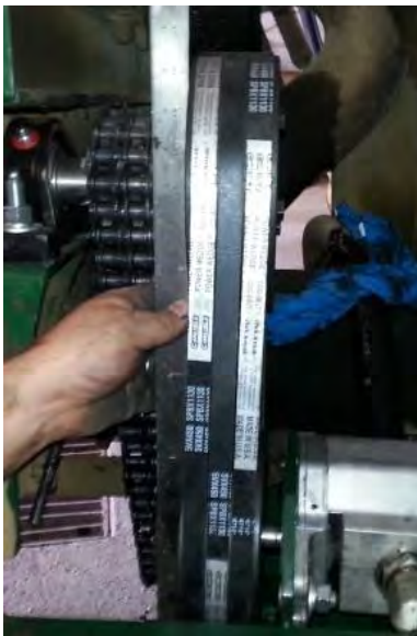
Figure 109a – Sheave Alignment (Use a Straight Edge if Possible).
