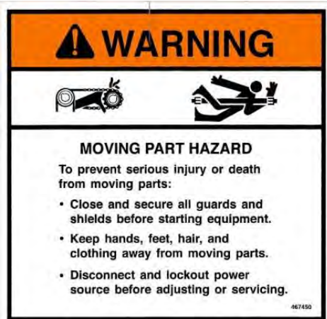
6. WARNING – Moving Part Hazard (467450)
