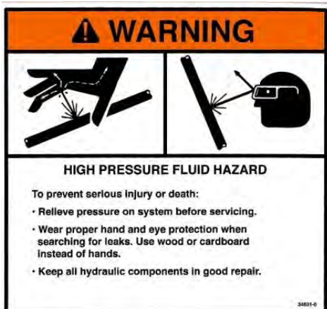
8. WARNING – High Pressure Fluid Hazard (346310)
