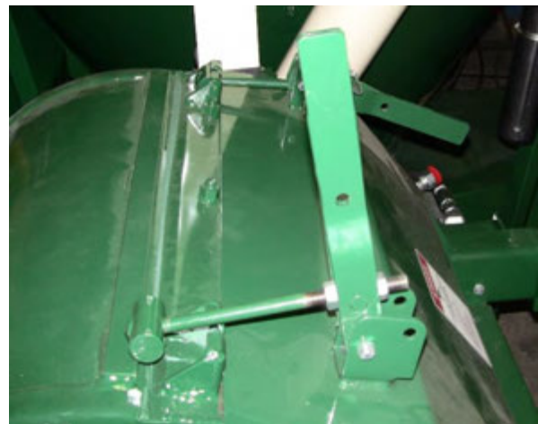
Figure 52 – Hammer Mill Door Pressure.
