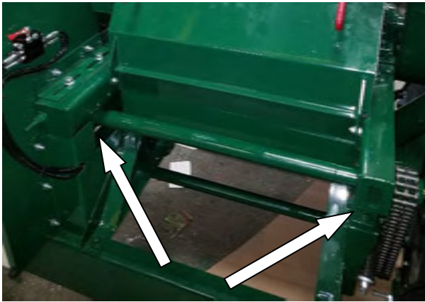
Figure 70 - Jack Shaft Front and Rear Bearings. Greased via the Remote Grease Block in Figure 69.
