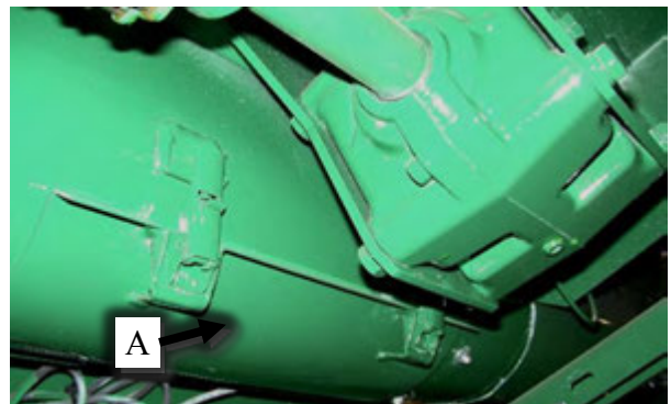
Figure 25 - Cleanout Door (A) Located Under Right Hand Side of Tank Assembly.
