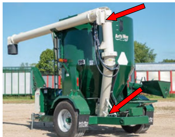
Figure 56 - Discharge Auger Drive Chain Locations (See Arrows).
