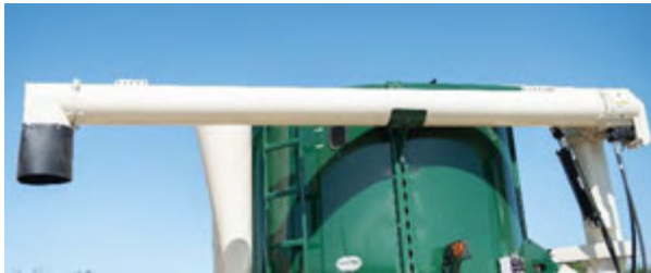
Figure 28 - Unloading Auger Positioning (Shown in Upper 60° to -11° Configuration).
