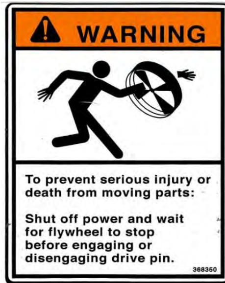
8. WARNING – Moving Flywheel Hazard (368350)
