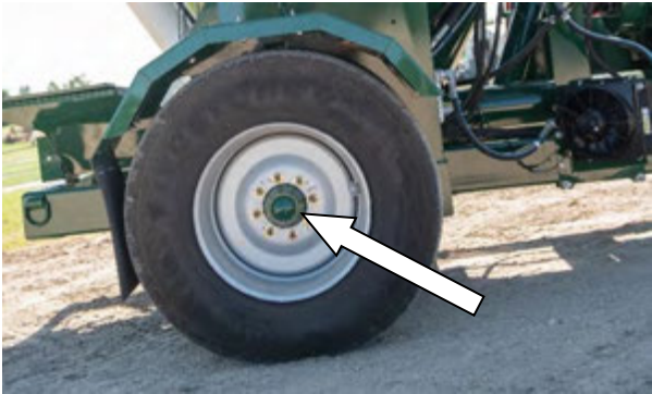
Figure 81 - Wheel Bearing Lubrication.
