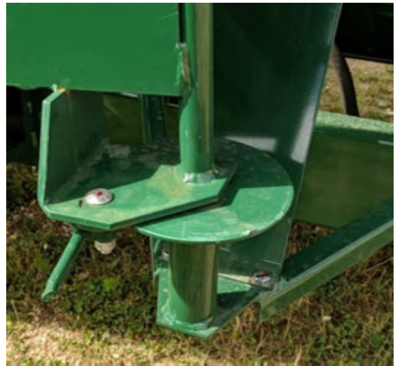
Figure 39 - Auger Feeder Swing Brake.
