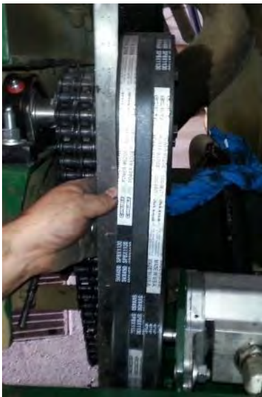
Figure 109a – Sheave Alignment (Use a Straight Edge).
