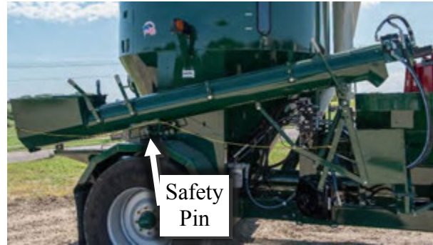
Figure 37 – Auger Feeder (Shown in Transport Position).
