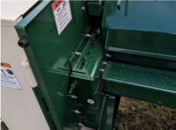
Figure 92, Detail B). Then relieve the belt tension by loosening the bolt (see Figure 92, Detail A) and move bearing mount and sheave.
