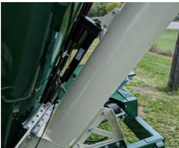
Figure 31 - Discharge Gate with Electric Actuator in Closed Position.
