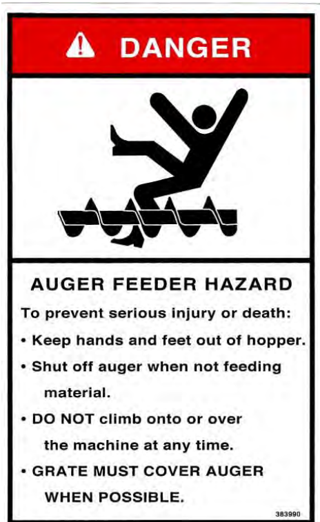
6. DANGER – Auger Feeder Hazard (383990)
