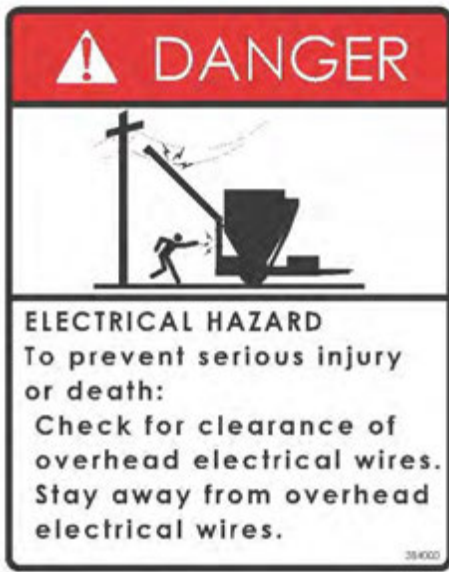
7. DANGER – Electrocutation Hazard (384000)
