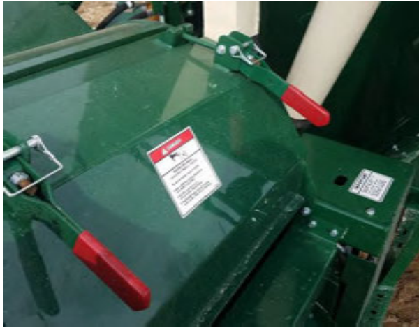
Figure 23 - Locking Pin and Latch on Hammer Mill Door.
