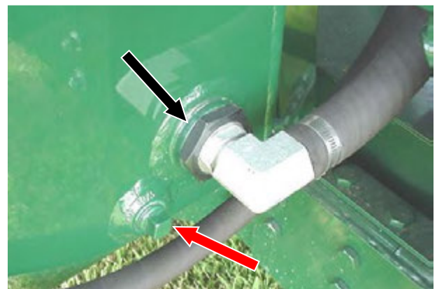
Figure 76 – Reservoir Strainer (Black Arrow) and Drain Plug at Front of Reservoir Tank (Red Arrow).
