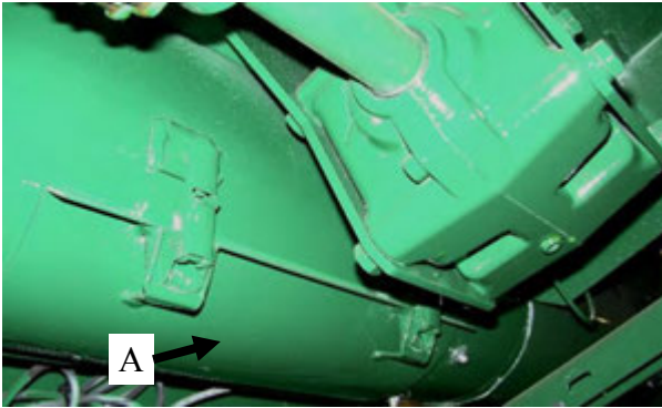
Figure 20 - Cleanout Door (A) Located Under Right Hand Side Of Tank Assembly.
