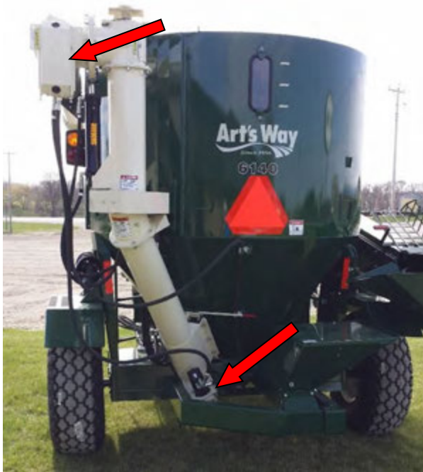
Figure 42 - Discharge Auger Drive Chain (See Arrows).
