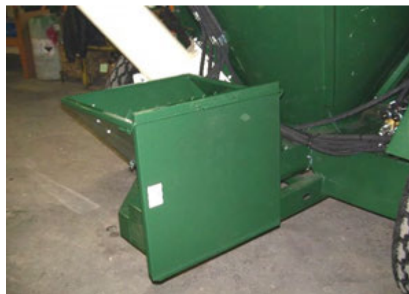
Figure 19 - Supplement Hopper Located on Center Rear Right Hand Side of Machine.
