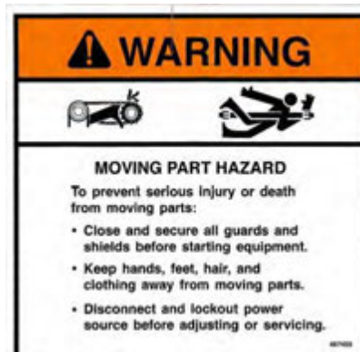
6. WARNING – Moving Part Hazard (467450)
