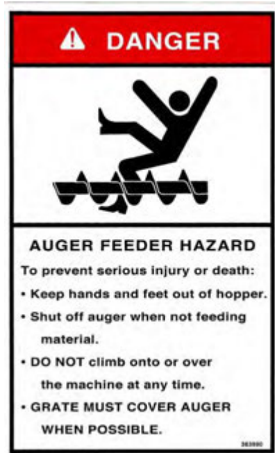
4. DANGER – Auger Feeder Hazard (383990)
