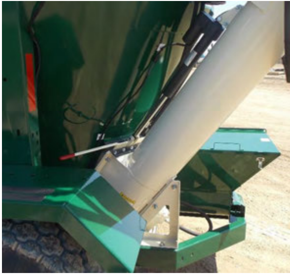
Figure 85 - Discharge Gate with Electric Actuator in closed position.
