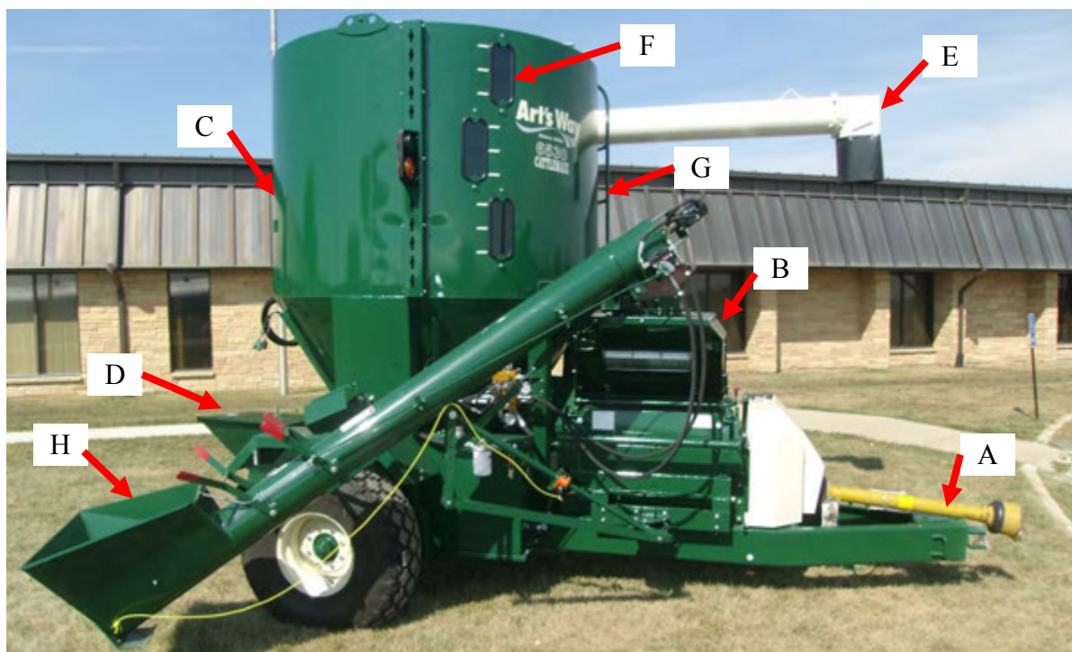
Figure 6 - Model 6140 CattleMaxx With Auger Feeder (A – PTO Driveline; B – Roller mill and Hopper; C – Mixing Tank; D – Supplemental Hopper; E – Discharge Auger; F – Viewing Windows; G – Ladder; H - Auger Feeder).
