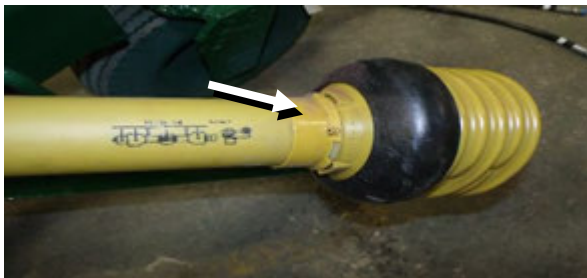
Figure 163 - Plastic Shaft Bearings (See Arrow).
