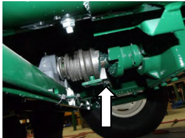
Figure 80 - Unloading Clutch Operation.
