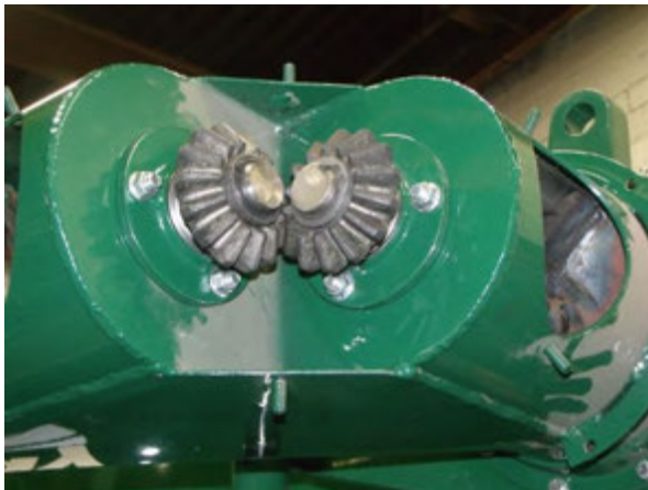
Figure 83 - Discharge Auger Bevel Gears, Outer Elbow (Shields Removed For Clarity).
