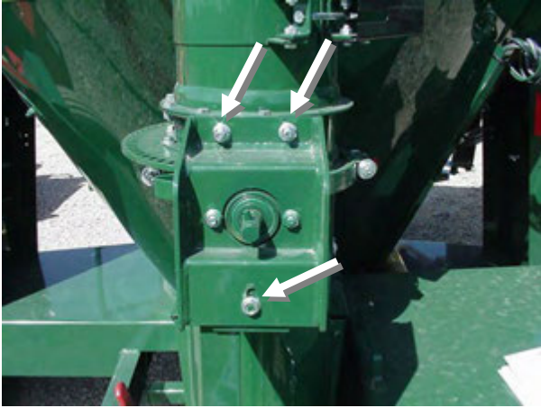
Figure 51 - Manual Unloading Auger Swing Crank Adjustment
