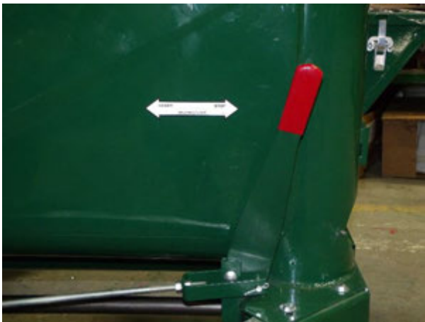
Figure 29 - Unloading Clutch Operation.
