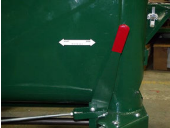
Figure 131 - Unloading Clutch Operation.
