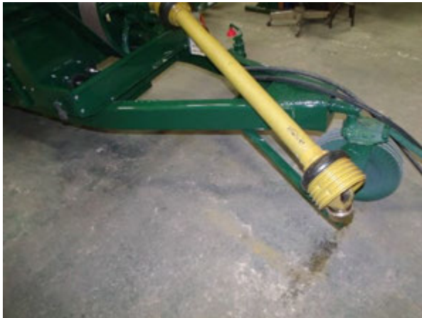
Figure 66 - PTO Driveline (Shield Removed For Clarity).
