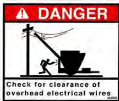
5. DANGER - Electrocutation Hazard (384000)
