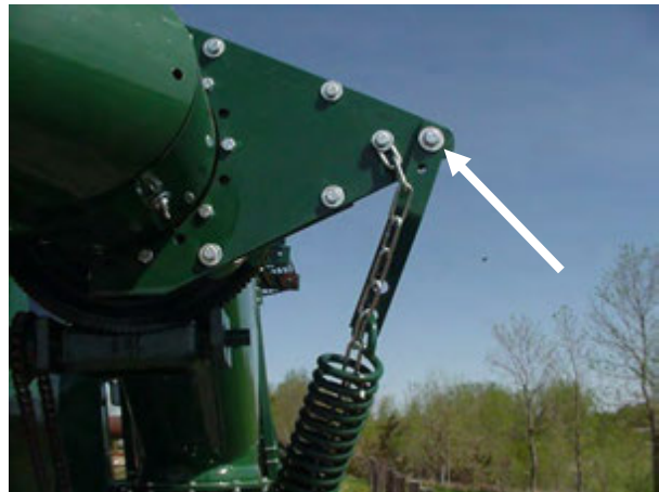
Figure 155 - Lift Assist Spring Adjustment Bolts
