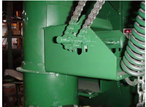
Figure 53 - Crank Shaft Chain Adjustment Bolts
