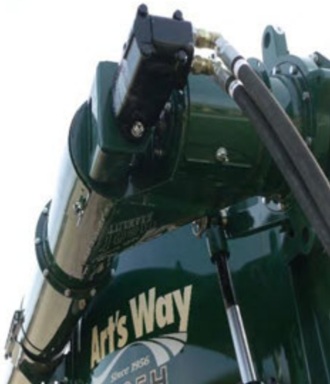
Figure 55 - Upper Discharge Motor (Unload)
