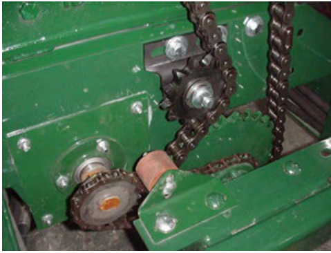
Figure 181 – Sprocket And Chain Alignment
