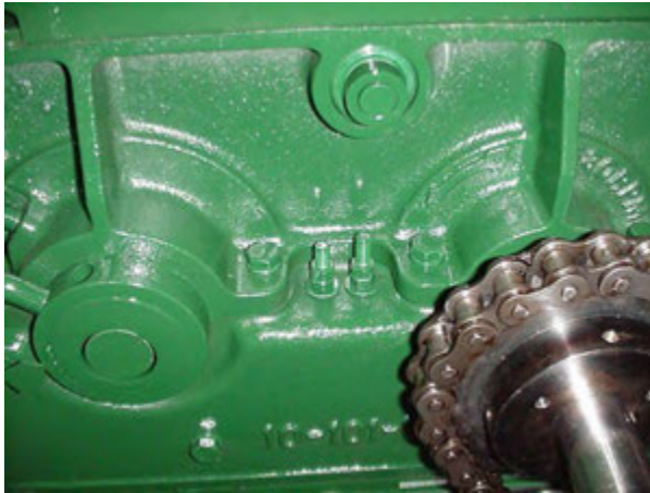
Figure 149 - Roll Scraper Adjustment Bolts
