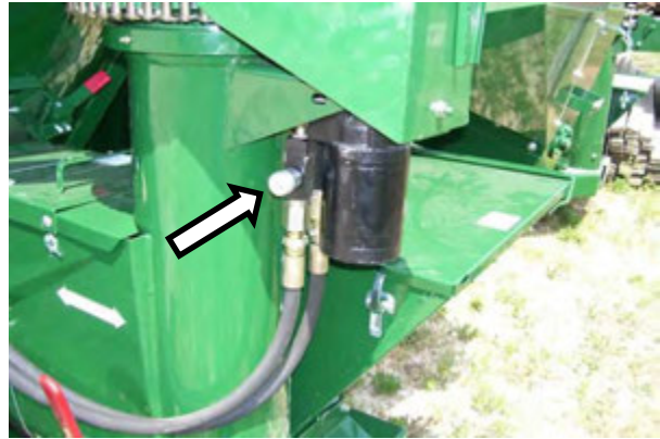
Figure 154 - Hydraulic Swing Flow Control Valves.
