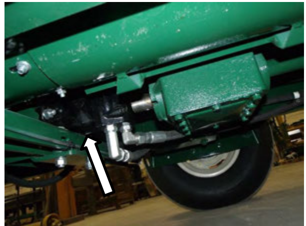
Figure 57 - Lower Discharge Motor (First Section)
