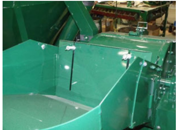
Figure 17 - Feed Gate At Throat Of The Hammermill.
