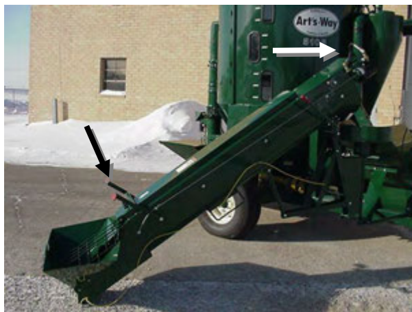
Figure 39 - Hydraulic auger feeder controls. (See arrows)
