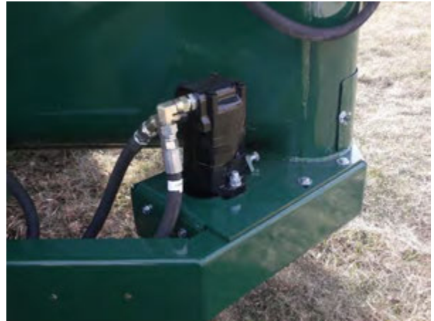
Figure 56 - Middle Discharge Motor (Vertical)
