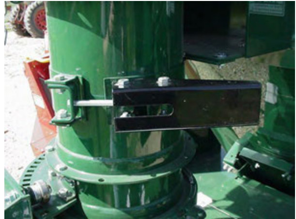
Figure 151 – Manual Brake Adjustment
