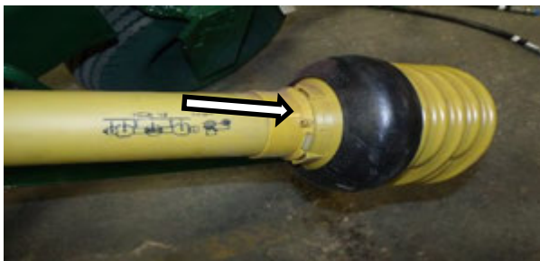
Figure 67 - Plastic Shaft Bearings (See Arrow).
