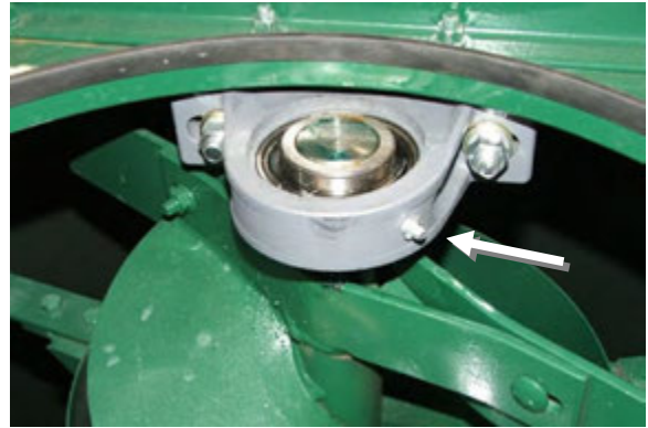
Figure 172 - Upper Vertical Mixing Auger Bearing.
