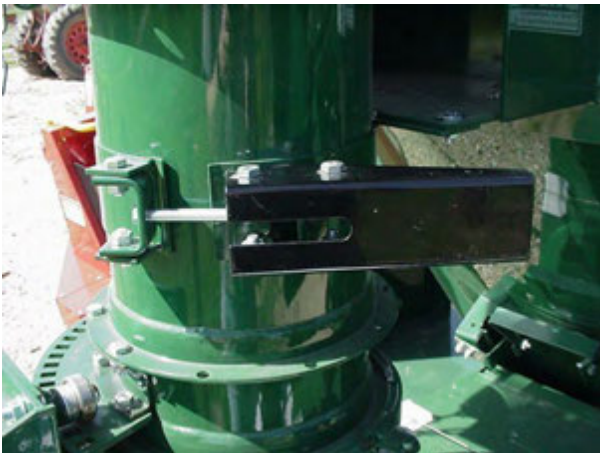
Figure 52 – Manual Brake Adjustment
