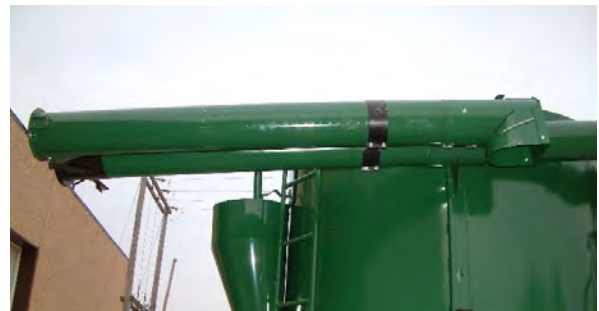
Figure 32 - Folding Auger Extension. (6' Extension shown)
