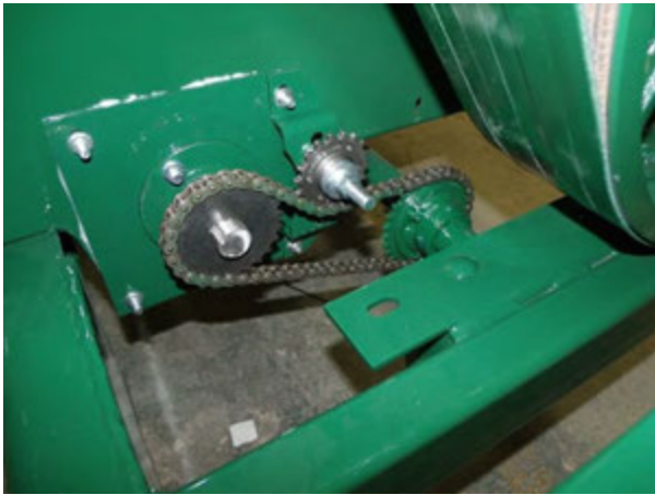
Figure 42 - Mill To Mixer Auger Drive Chain.
