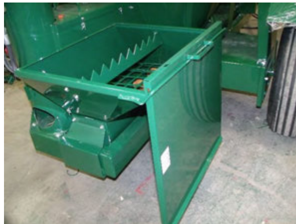
Figure 122 - Supplement Hopper On Right-Hand Side Of Machine.
