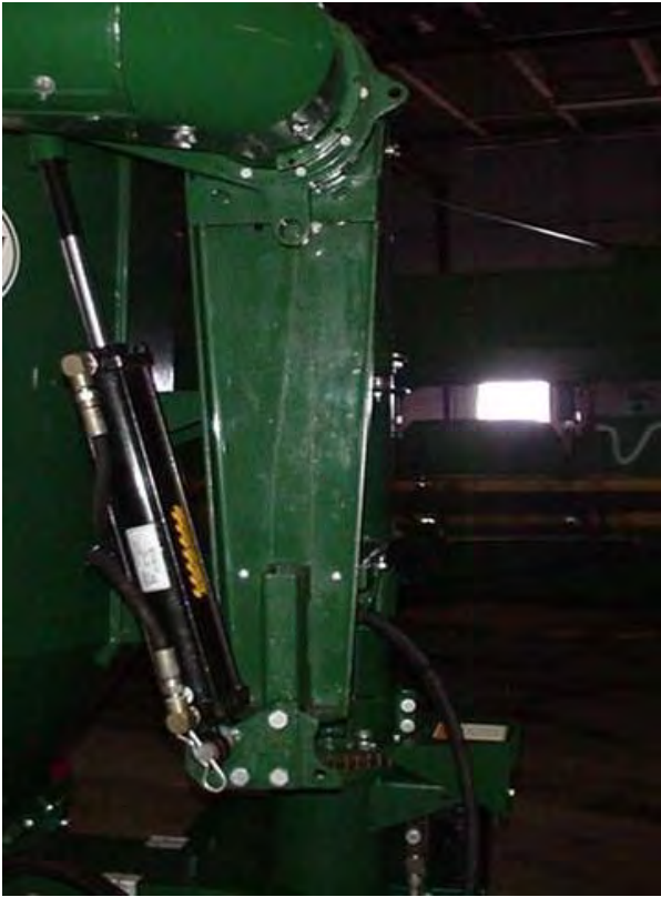
Figure 58 - Discharge Auger Lift Cylinder Adjustment.
