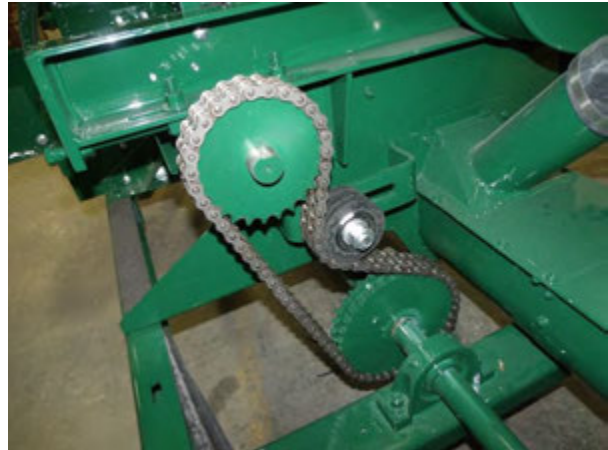
Figure 44 - Drive Chain Adjustment (Shields Removed For Clarity).
