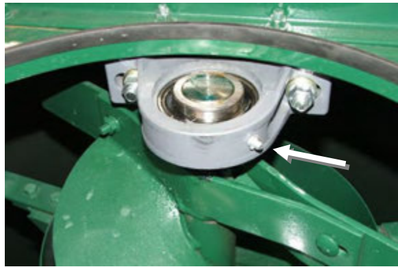
Figure 79 – Upper Vertical Mixing Auger Bearing.
