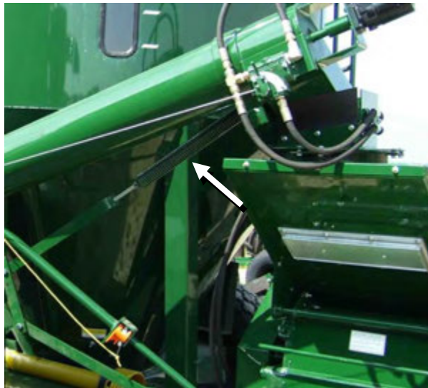
Figure 139 – Auger Feeder Counter Balance Spring
