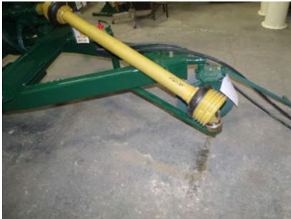
Figure 162 - PTO Driveline (Shield Removed For Clarity).
