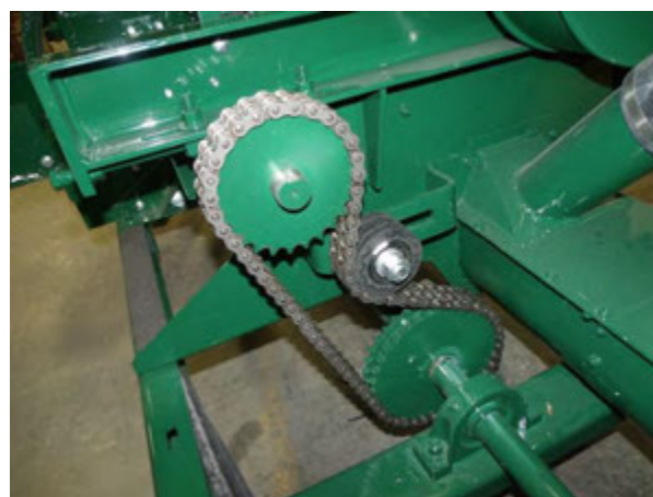
Figure 90 – Jack Shaft to Mixing Auger Sprockets (Shields Removed For Clarity).
