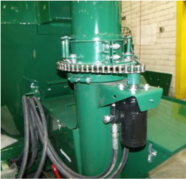
Figure 153 - Hydraulic Swing Adjustment (Shields Removed For Clarity).
