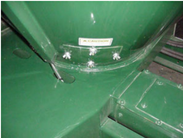
Figure 123 - Tank Cone Clean-Out Door On Right-Hand Side.
