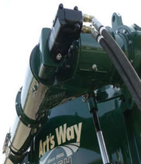
Figure 156 - Upper Discharge Motor (Unload)
