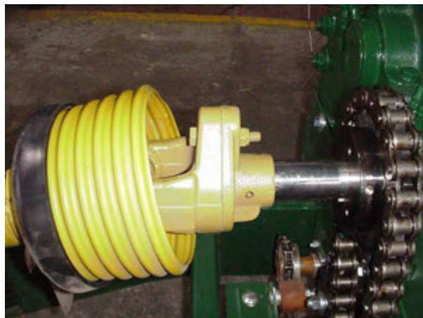
Figure 118 - PTO Driveline Shear Clutch
