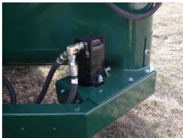
Figure 157 - Middle Discharge Motor (Vertical)
