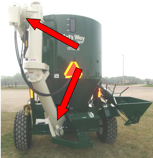
Figure 52 – Discharge Auger Drive Chain Locations (see arrows).
