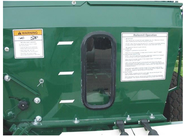
Figure 42 - Hopper Inspection Window.
