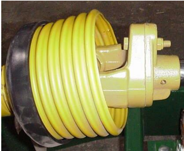
Figure 18 - PTO Driveline Shear Clutch
