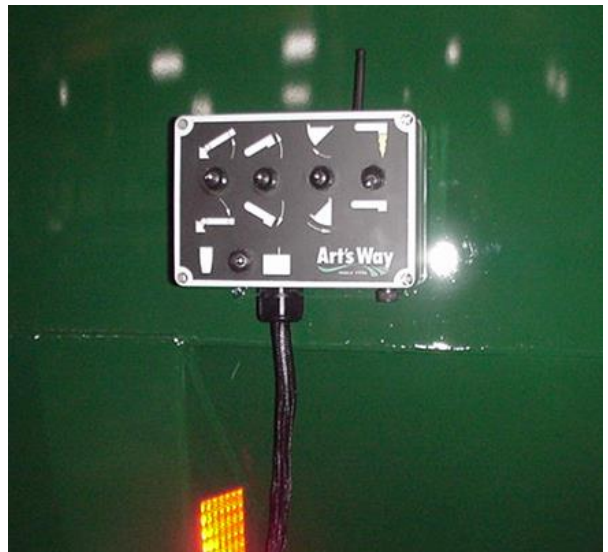
Figure 89 – Complete Control Box with Internal Receiver Mounted on Left Rear Side of Tank.
