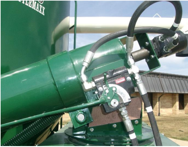
Figure 41 - Auger Feeder Flow Control Valve (Shown In "OFF" Position).
