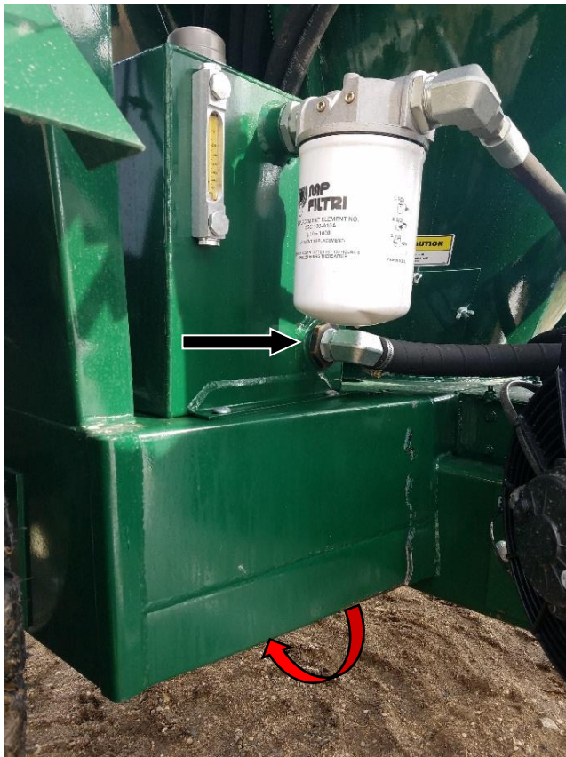
Figure 97 – Reservoir Strainer (Black Arrow) and Drain Underneath Reservoir Tank Base (Red Arrow).
