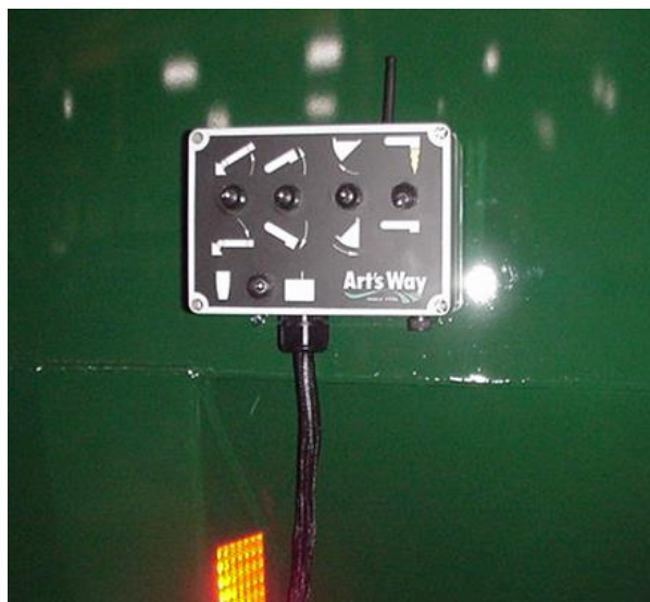
Figure 85 – Complete Control Box with Internal Receiver.
