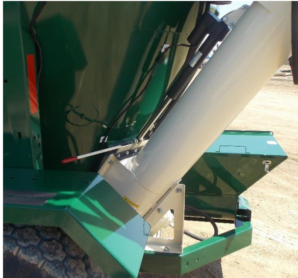
Figure 30 - Discharge Gate with Electric Actuator in Closed Position.
