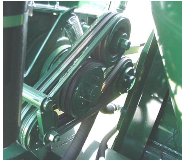
Figure 63 – Roller mill Belt Drive (Shield Removed for Clarity).
