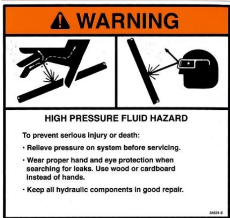
8. WARNING – High Pressure Fluid Hazard (346310)
