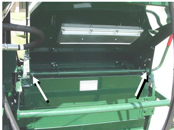
Figure 61 - Grain Control Gate Lubrication (2-Zerks and Slide Guides).
