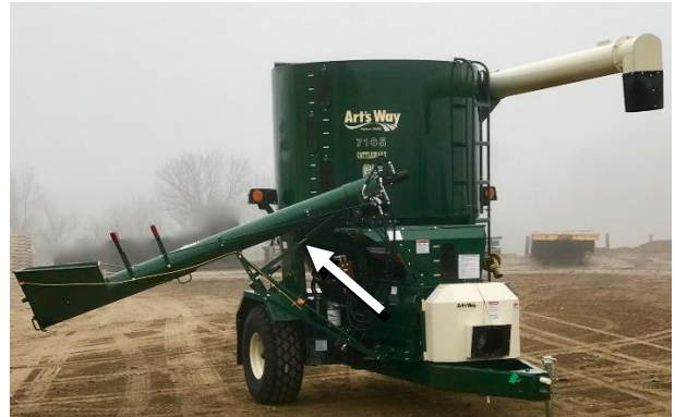
Figure 39 – Auger Feeder Counter Balance Spring
