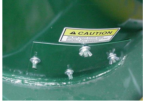
Figure 23 - Tank Cone Clean-Out Door (Left-Hand Side Shown).
