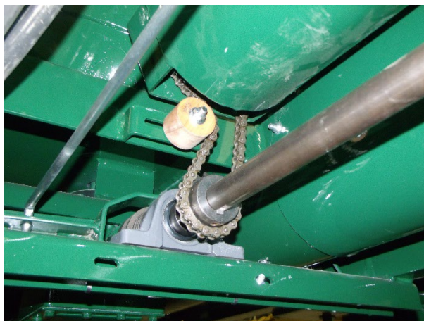
Figure 43 - Discharger Auger Drive Chain (Shields Removed for Clarity).
