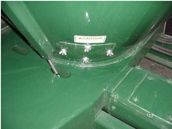
Figure 123 - Tank Cone Clean-Out Door On Right-Hand Side.
