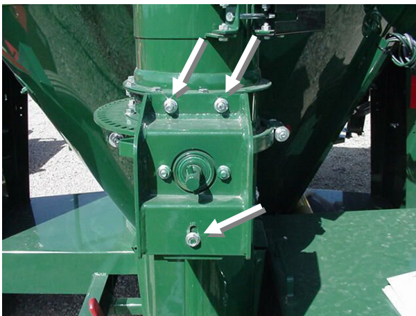
Figure 150 - Manual Unloading Auger Swing Crank Adjustment
