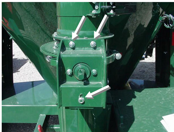
Figure 51 - Manual Unloading Auger Swing Crank Adjustment
