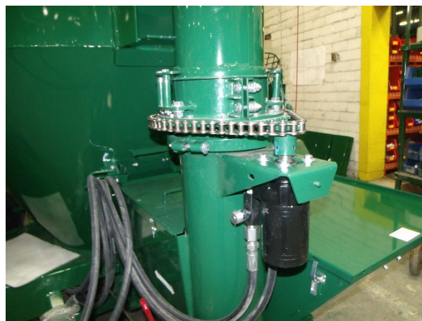
Figure 60 - Hydraulic Swing Adjustment (Shields Removed For Clarity).
