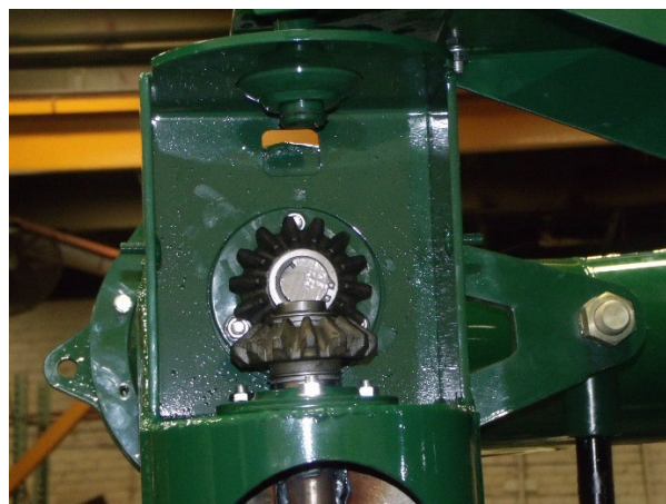
Figure 176 - Discharge Auger Bevel Gears, Inner Elbow (Shields Removed For Clarity).
