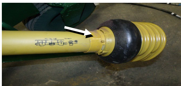
Figure 163 - Plastic Shaft Bearings (See Arrow).
