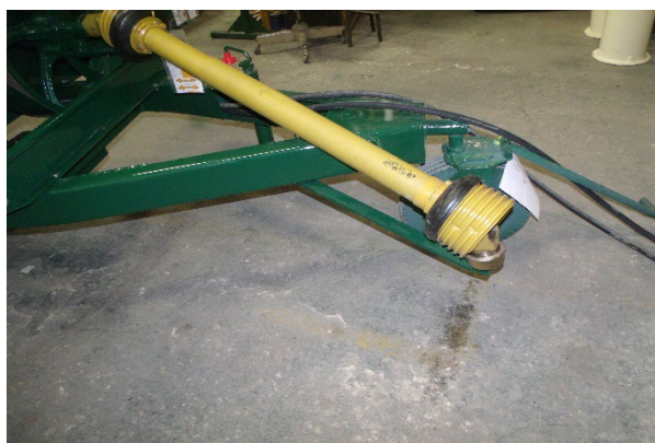
Figure 9 - PTO Driveline Storage Bracket.
