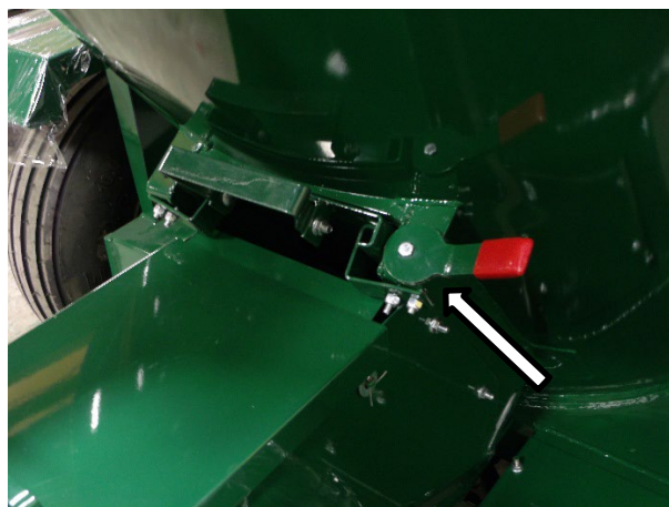
Figure 30 - Unloading Door (A - Eccentric Lock).
