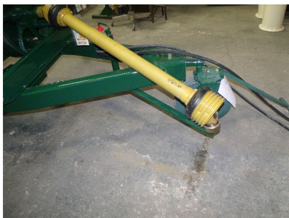
Figure 162 - PTO Driveline (Shield Removed For Clarity).
