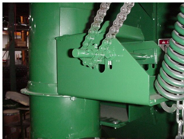
Figure 53 - Crank Shaft Chain Adjustment Bolts
