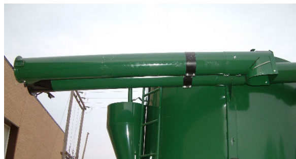
Figure 32 - Folding Auger Extension. (6' Extension shown)
