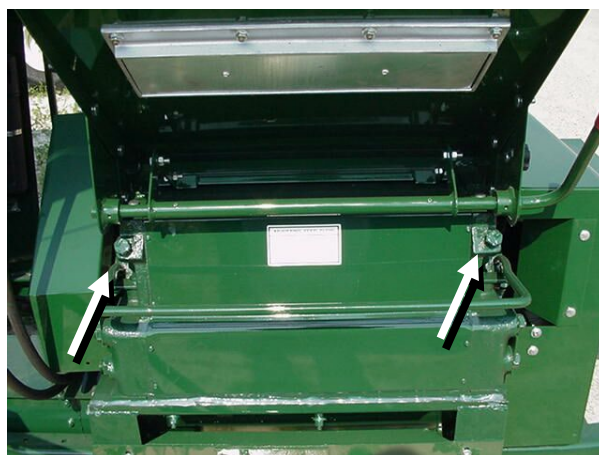
Figure 164 - Grain Control Gate Lubrication (2 Zerk and Slide Guides).
