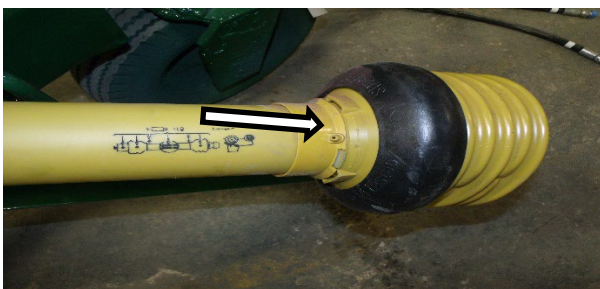
Figure 67 - Plastic Shaft Bearings (See Arrow).
