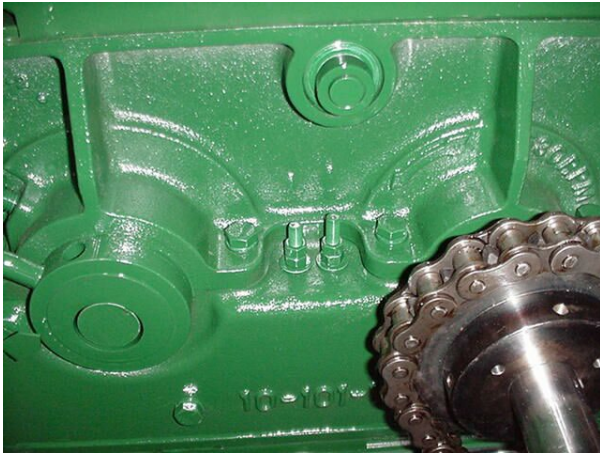
Figure 149 - Roll Scraper Adjustment Bolts
