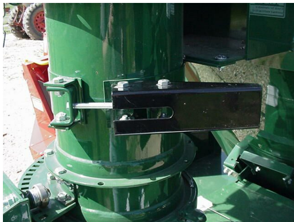
Figure 52 – Manual Brake Adjustment
