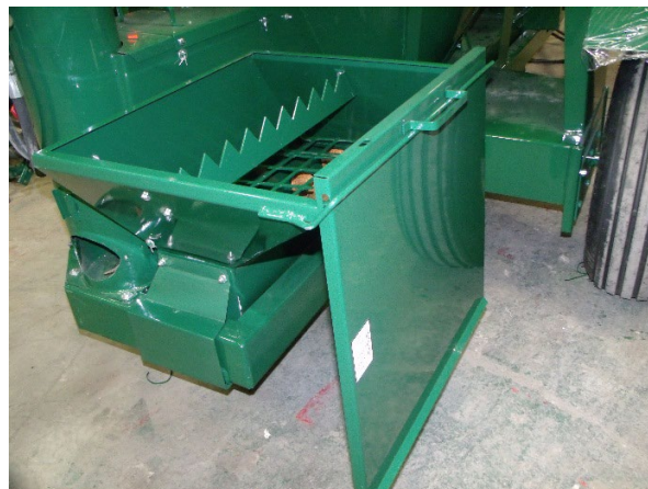
Figure 122 - Supplement Hopper On Right-Hand Side Of Machine.
