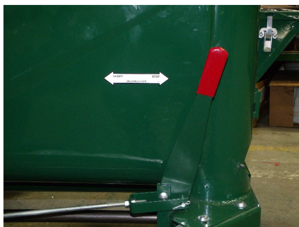
Figure 29 - Unloading Clutch Operation.
