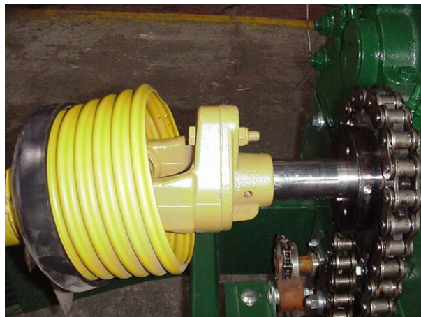
Figure 118 - PTO Driveline Shear Clutch
