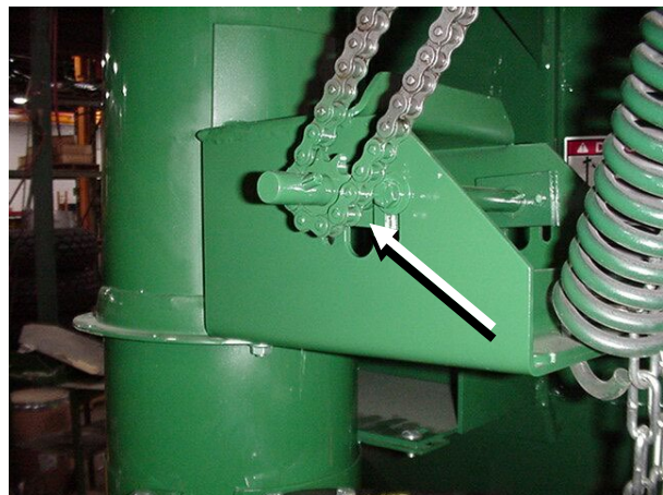
Figure 152 - Crank Shaft Chain Adjustment Bolts
