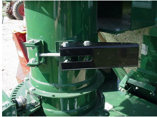
Figure 151 – Manual Brake Adjustment
