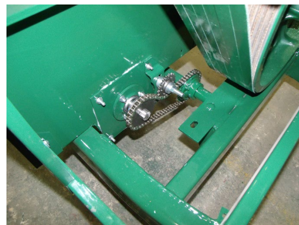
Figure 91 – Mill To Mixer Sprocket (Shields Removed For Clarity).
