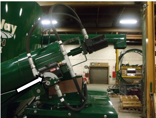
Figure 40 - Hydraulic Auger Feeder Control. (See Arrow)
