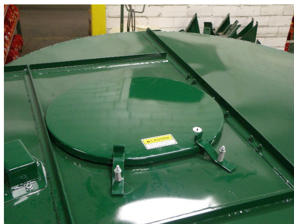
Figure 126 - Spring Loaded Tank Lid.
