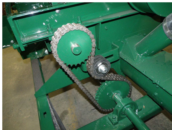
Figure 44 - Drive Chain Adjustment (Shields Removed For Clarity).
