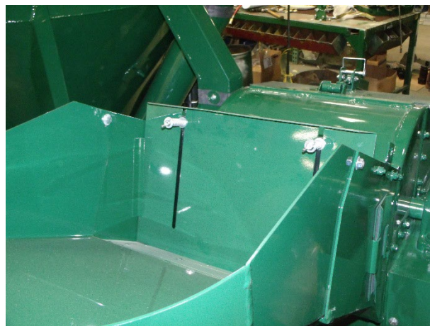
Figure 17 - Feed Gate At Throat Of The Hammermill.
