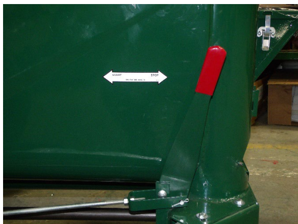
Figure 131 - Unloading Clutch Operation.
