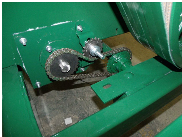
Figure 42 - Mill To Mixer Auger Drive Chain.
