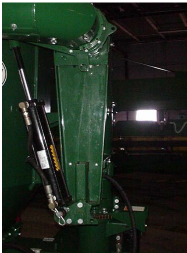
Figure 58 - Discharge Auger Lift Cylinder Adjustment.
