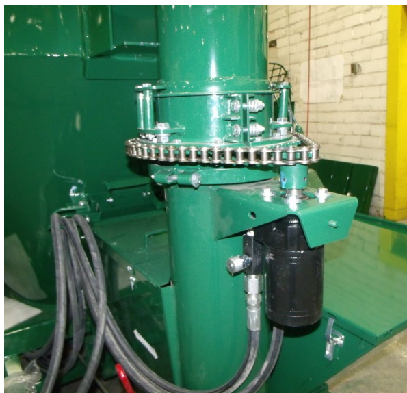
Figure 153 - Hydraulic Swing Adjustment (Shields Removed For Clarity).
