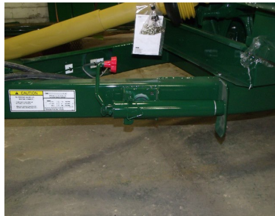
Figure 12 - Jack In Transport Position
