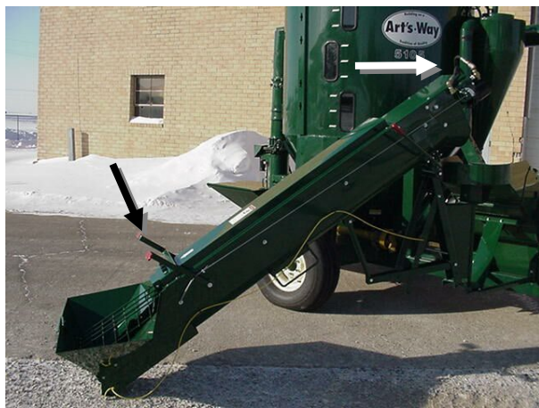
Figure 39 - Hydraulic auger feeder controls. (See arrows)
