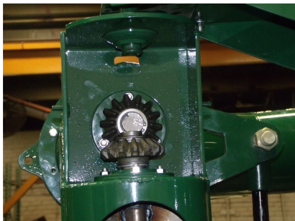
Figure 82 - Discharge Auger Bevel Gears, Inner Elbow (Shields Removed For Clarity).
