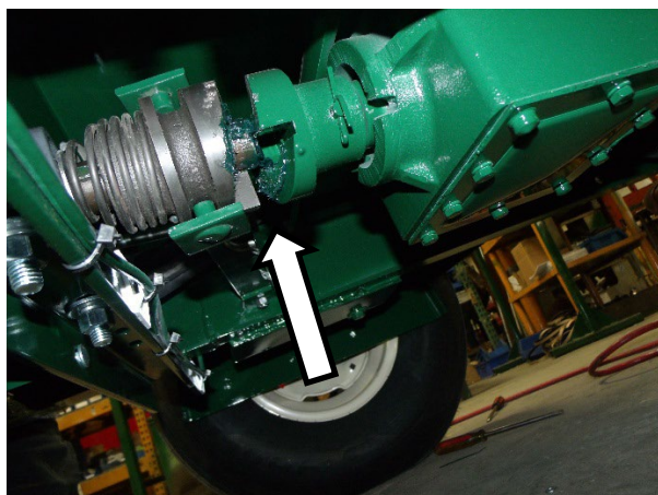
Figure 174 - Unloading Clutch Operation.
