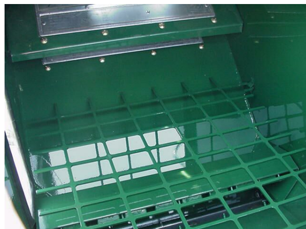
Figure 148 - Removing Magnet To Check Roll Spacing.
