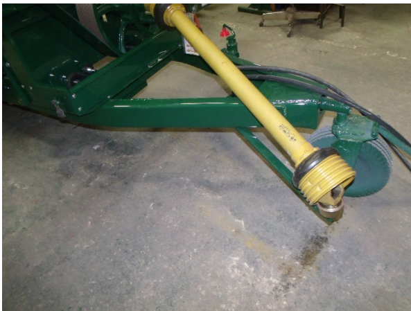
Figure 66 - PTO Driveline (Shield Removed For Clarity).
