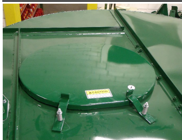
Figure 24 - Spring Loaded Tank Lid.
