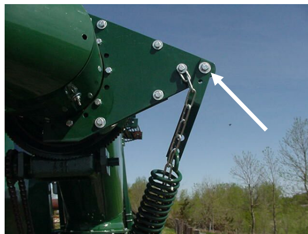
Figure 155 - Lift Assist Spring Adjustment Bolts
