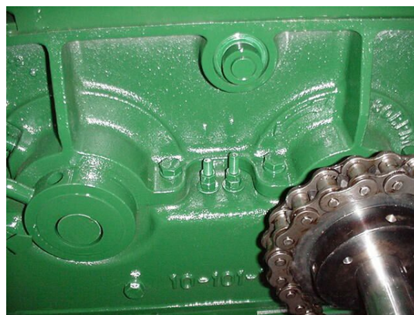
Figure 38 - Roll Scraper Adjustment Bolts
