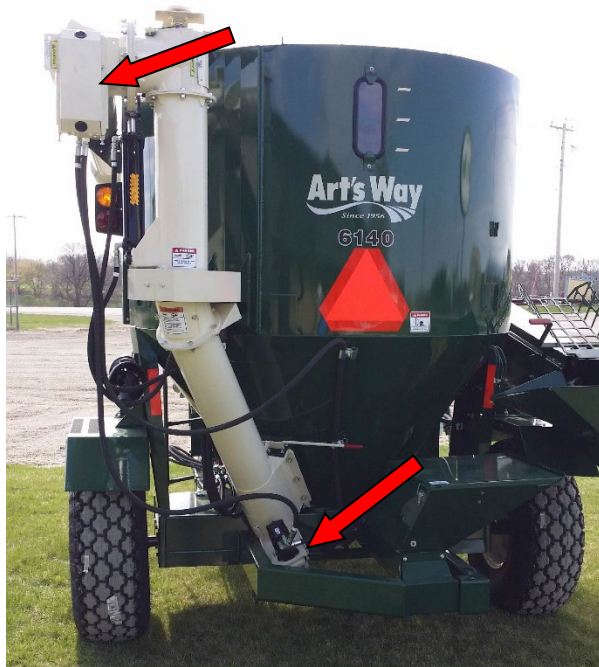
Figure 42 - Discharge Auger Drive Chain (See Arrows).
