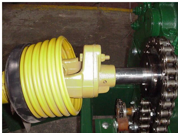
Figure 15 - PTO Driveline Shear Clutch
