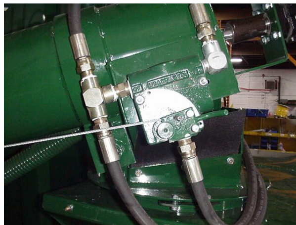
Figure 33 - Hydraulic Auger Feeder Controls (Shown in On).
