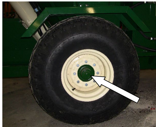
Figure 63 - Wheel Bearing Lubrication.
