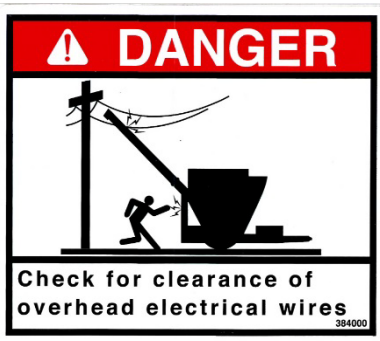
5. DANGER – Electrocutation Hazard (384000)
