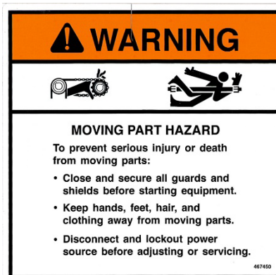
6. WARNING – Moving Part Hazard (467450)
