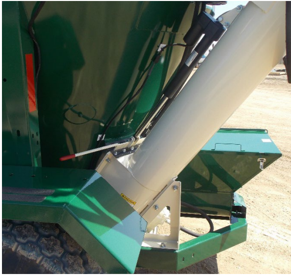
Figure 25 - Discharge Gate with Electric Actuator in closed position.
