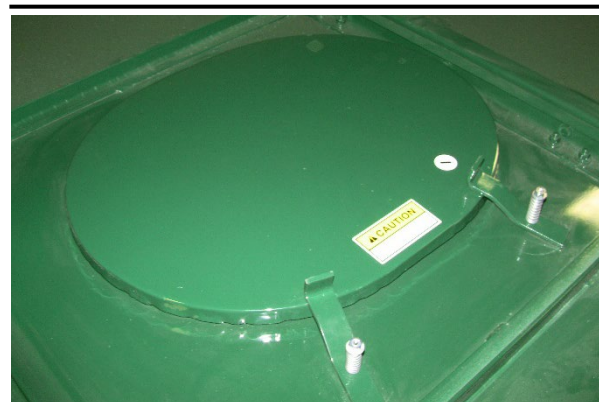
Figure 22 - Spring Loaded Tank Lid.
