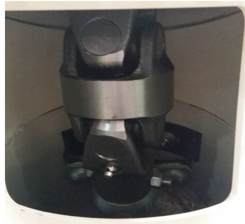
Figure 61 – Discharge U-Joint (Door/flighting Removed for Clarity).
