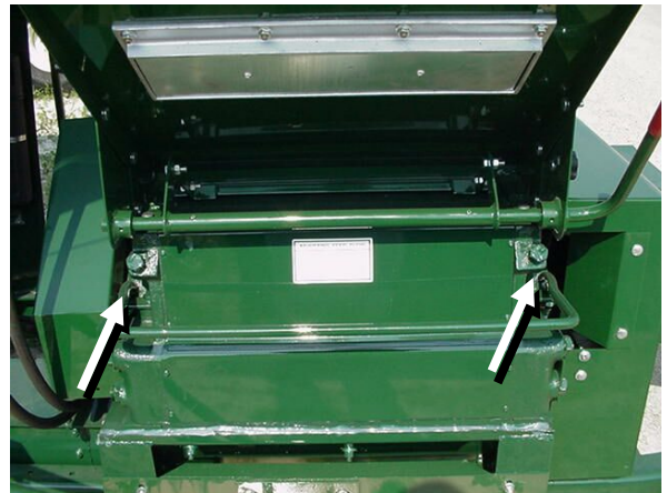
Figure 49 - Grain Control Gate Lubrication (2 Zerks and Slide Guides).
