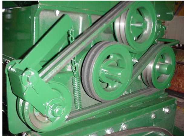
Figure 35 - Drive Chain Adjustment (Shields Removed For Clarity).
