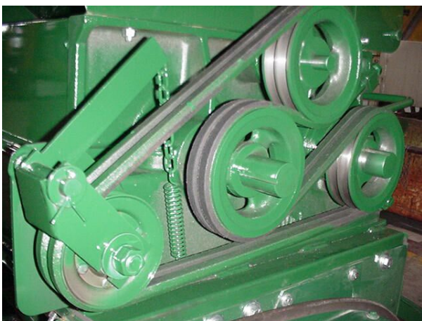
Figure 51 – Roller mill Belt Drive
