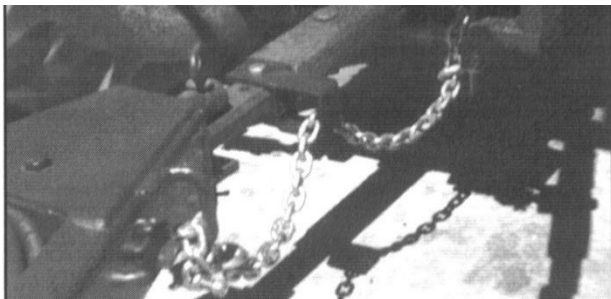
Figure 11 - Grinder Attached To The Tractor With Safety Chain.
