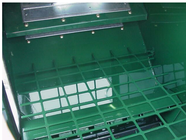
Figure 37 - Removing Magnet To Check Roll Spacing.
