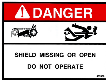
2. DANGER - Shield Missing (467430)
