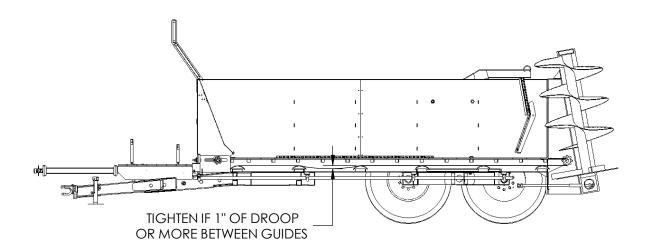
If apron is loose, remove one link from each side of that apron chain assembly and readjust to tension as shown. **CAUTION:** Over tightening can cause premature failure of the drive components. Check tension before operating. Re-tension if nessasary.
