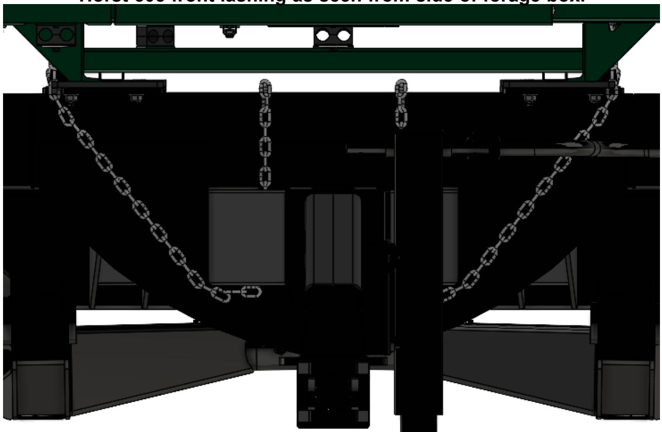
Horst 505 front lashing as seen from front of forage box.
